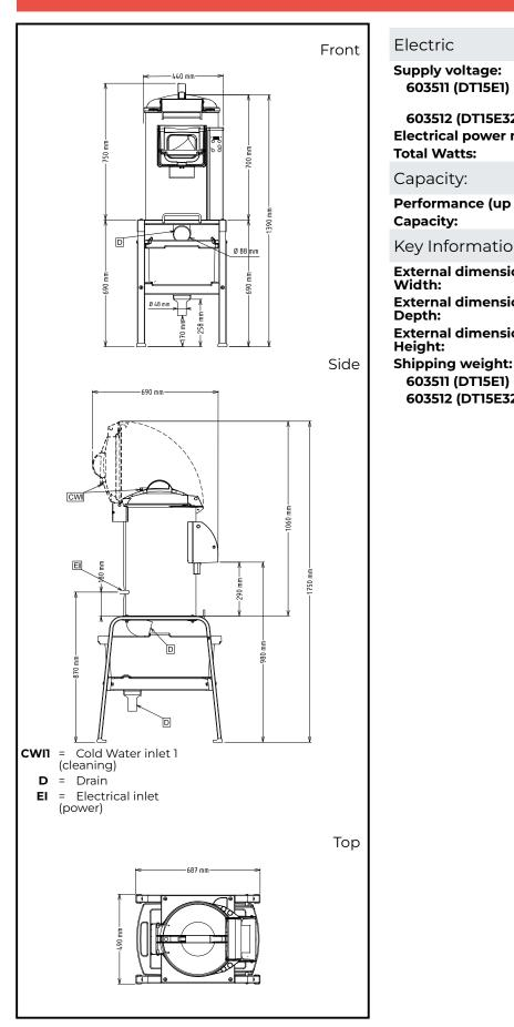
Electric Supply voltage: 603511 (DT15E1) 220-240 V/1N ph/50/60 Hz 200-240/380-440 V/3 603512 (DT15E324) ph/50/60 Hz Electrical power max: 0.37 kW 0.37 kW **Total Watts:** Capacity: Performance (up to): 240 kg/hour Capacity: 15 litres Key Information: External dimensions, Width: 440 mm External dimensions, 690 mm Depth: External dimensions,
